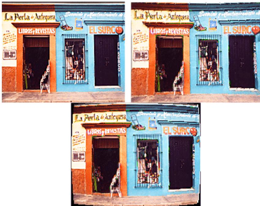
Fig. 5: Distortions in an actual object. From left to right: the original image; with a 10% pincushion-shaped distortion; with a 10% barrel-shaped distortion
