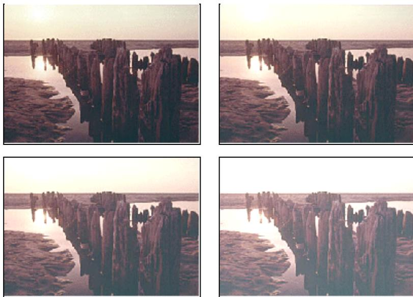
Fig. 8 Various stray light ratios in a picture. From upper left to lower right: original image, 6%, 12%, and 24%.
